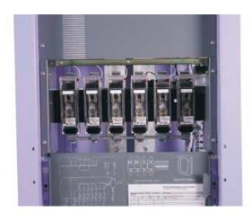
The Intergy DCF range of DC distribution modules provide protection for communications loads up to 2520A, using HRC type fuses in sizes from DIN00 to DIN3.
